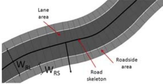
Fig. 4. Road shape model. The model consists in defining the width of the lane ( $W_{RL}$ ) and the width of two roadsides ( $W_{RS}$ ) perpendicular to the direction of each road segment defining the road skeleton.
