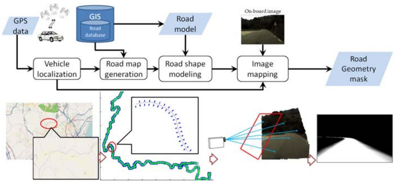
Fig. 2. Block-diagram of the algorithm for computing the road geometry using geographical information.
